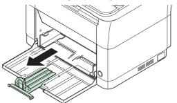
When using A6 paper, attach the stopper.
